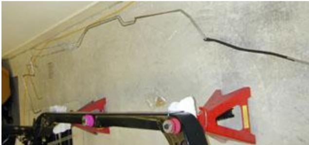
**Step 4.** With the protective caps in place, route the new lines into place on the car. The end caps protect the threads and prevent dirt from entering the lines. If you have new clips, install them in the exact position of the original clips. New clips are available from  for all common applications. Carefully route the new lines in the line clips and start the bolts in the clips, but do not completely tighten the lines or the clips.
