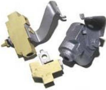
**Step 3.** In some cases, you will be re-using the original brake distribution block, proportioning valve, or other blocks that are not available new. These blocks should be cleaned and inspected before reassembly. Valves are available for all common cars on the [web site](#).
